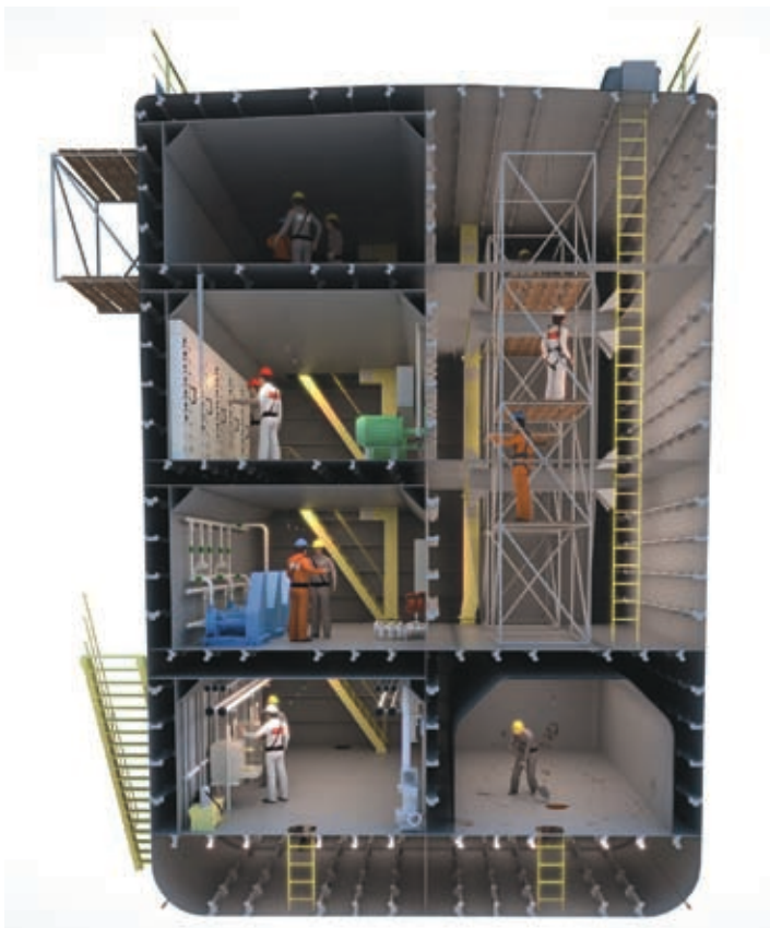
The new Integrated Safety Training Complex features a six level Mid-Ship Safety Module
