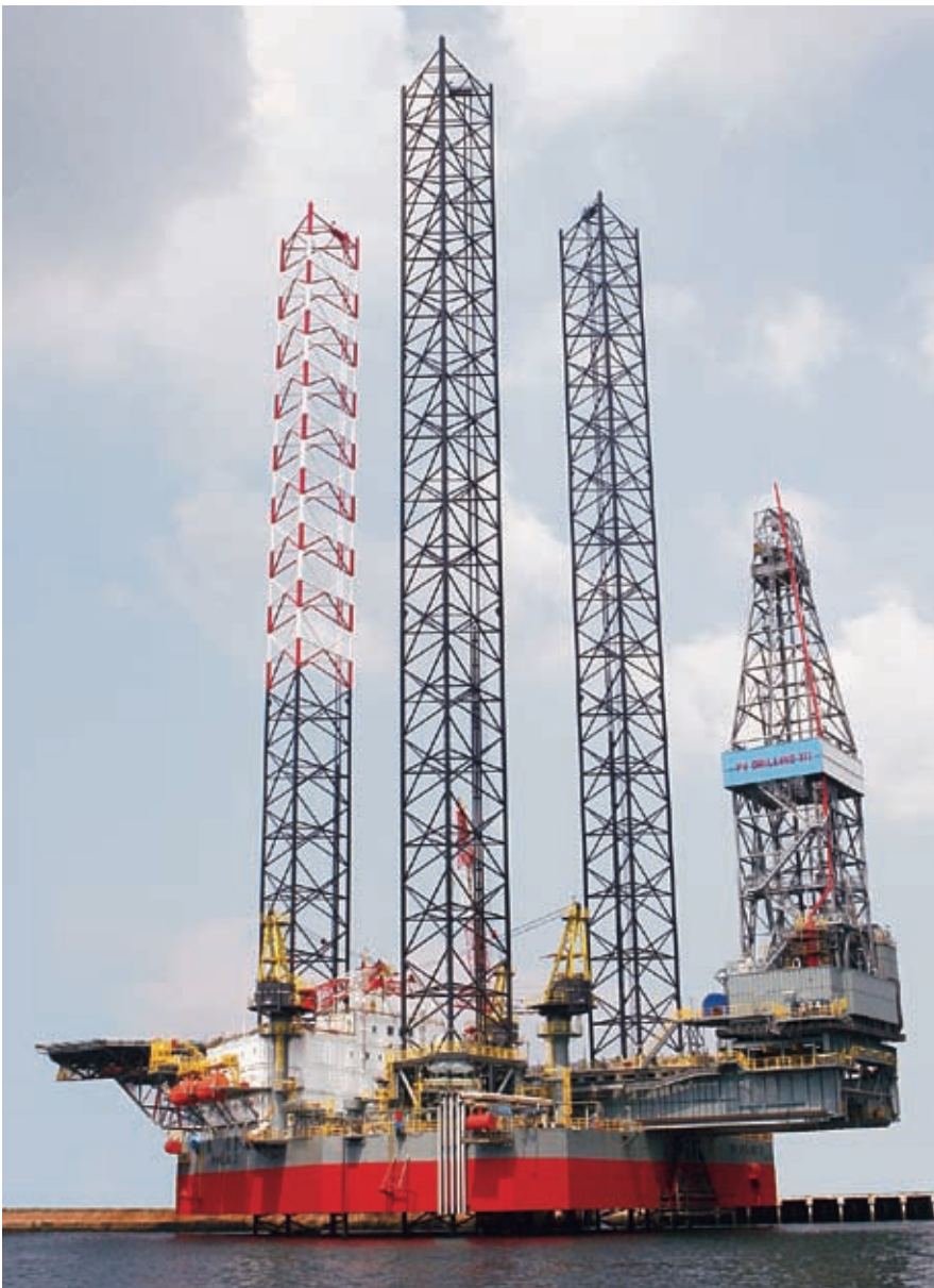
PV Drilling III completes the series of three KFELS B Class jackup rigs ordered by PV Drilling since 2005
