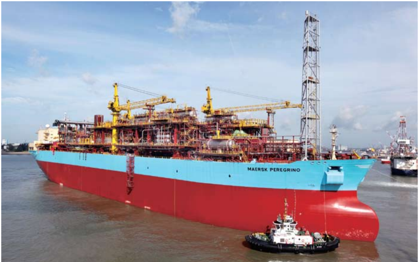
Maersk Peregrino was converted to meet Maersk FPSOs' stringent requirements which will prepare her to handle the heavy crude oil of the Peregrino field in offshore Brazil
