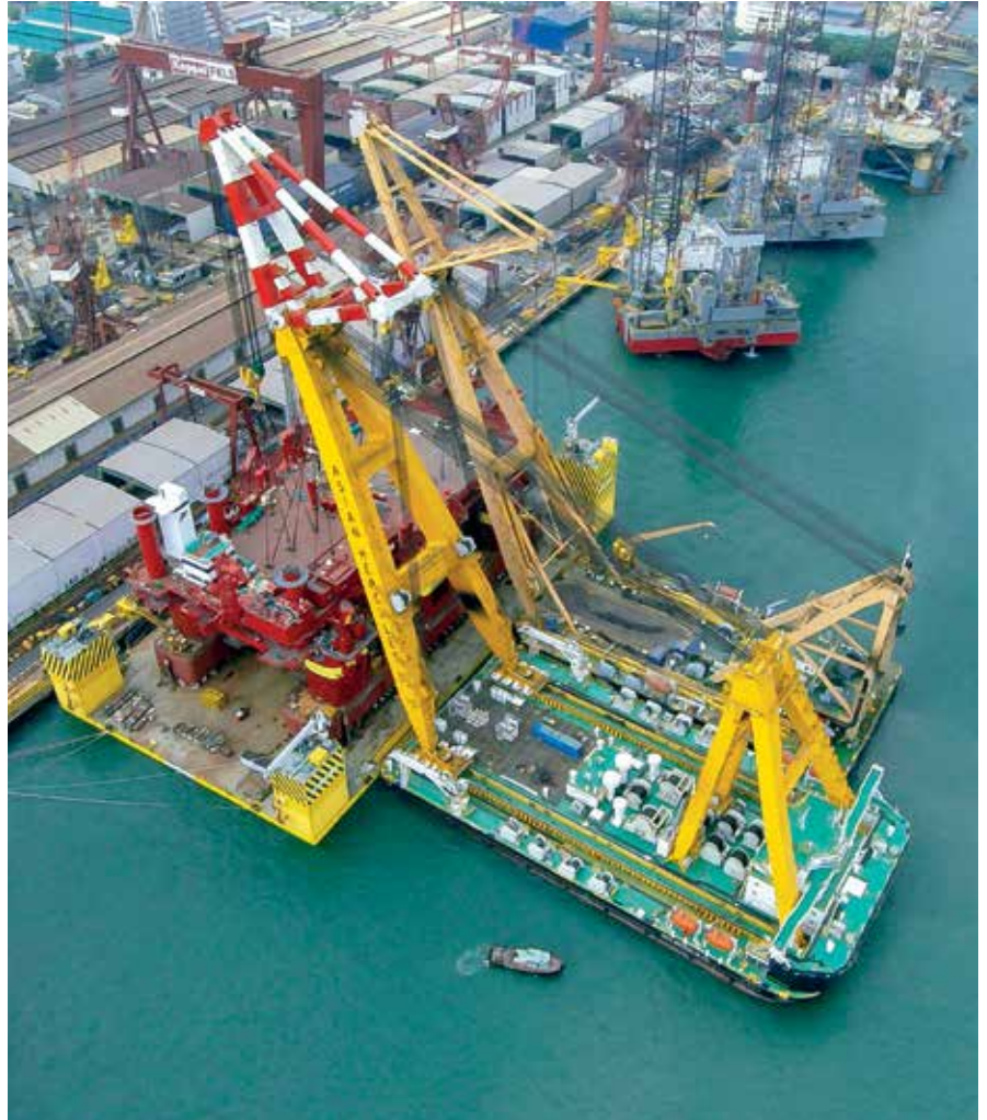
Asian Hercules III's first job was a tandem lift with Asian Hercules II for the 5,300-tonne upper hull of an accommodation semisubmersible
