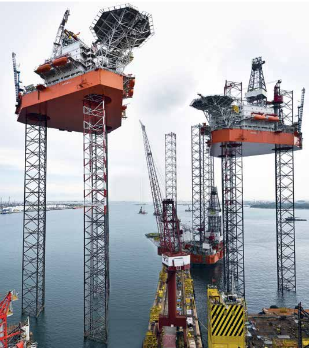
Keppel FELS has delivered CANTARELL I and CANTARELL II to Grupo R. Built to Keppel's proprietary KFELS B Class design, the rigs will be chartered to PEMEX for operations in the Cantarell oil field in offshore Mexico
