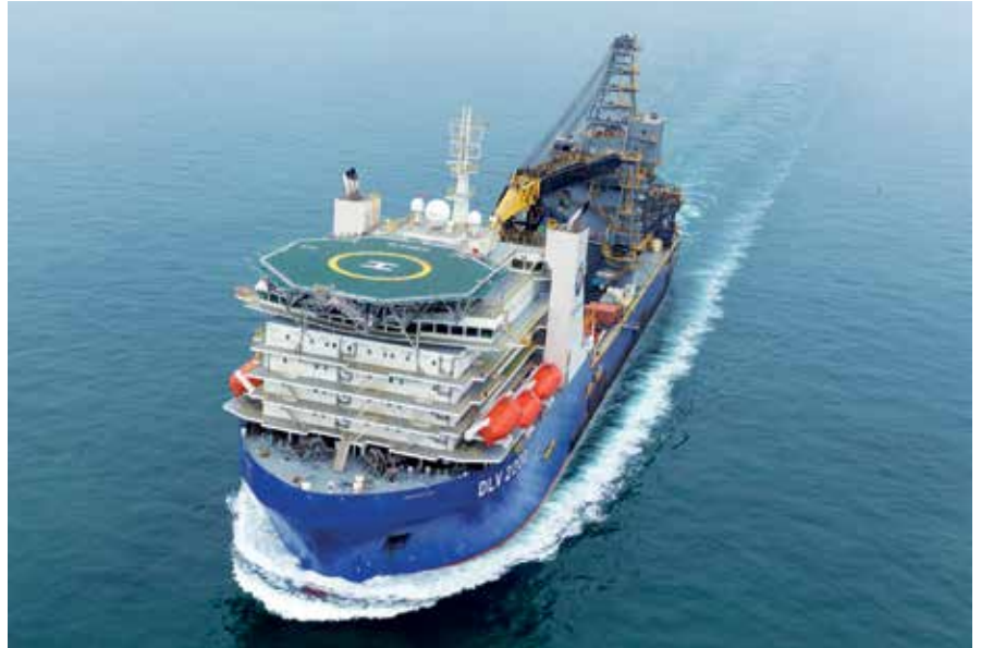
DLV 2000 is a high-specification deepwater derrick lay vessel built to Keppel's proprietary design. DLV 2000 will be deployed to operate in the INPEX Ichthys Liquefied Natural Gas project in offshore Western Australia
