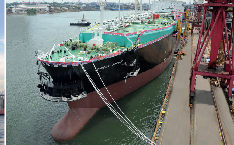
Floating Storage Unit (FSU) converted for Malaysia's first regasification terminal
