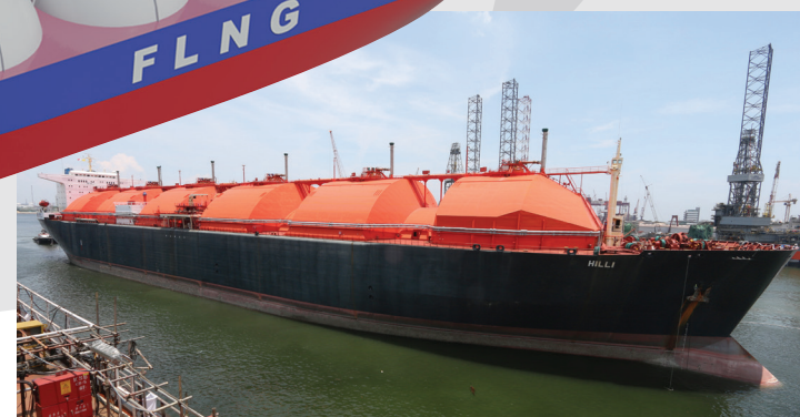
Moss-type LNG carrier, the HILLI, undergoing the world's first conversion into a FLNG facility by Keppel
