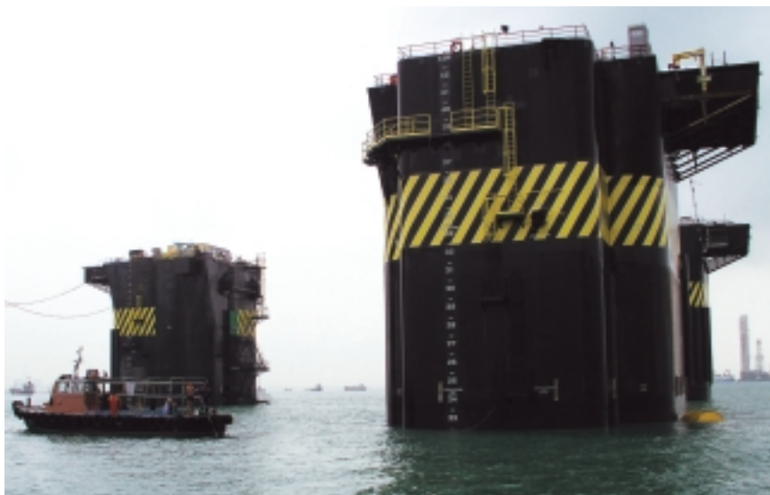
P-52 successfully completes the submergence trial (above and below right) and is towed back to Keppel FELS in preparation to depart for Keppel FELS Brasil (below)
