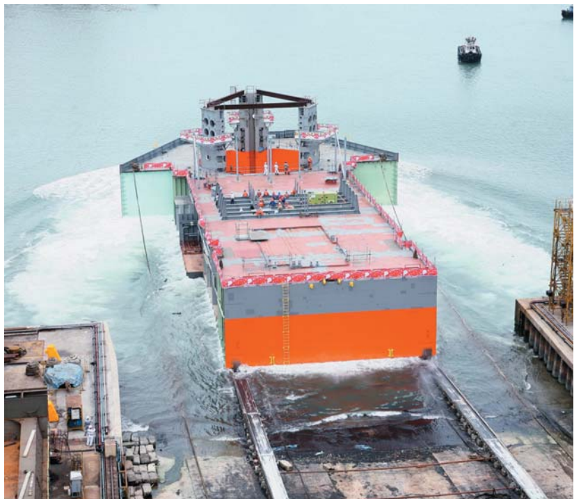
Virtue 1 launches into the next phase of construction as its centre hull strip heads for the Admiral dock
