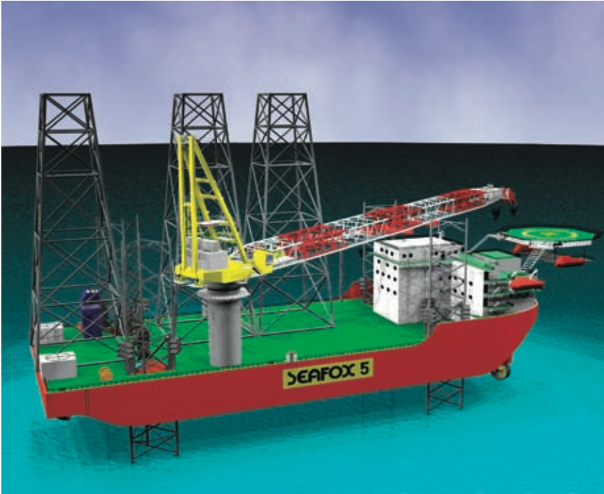
Keppel FELS's new multi-purpose self-elevating platform, KFELS MPSEP, is set to redefine the way in which offshore wind farms are installed and maintained across the world
