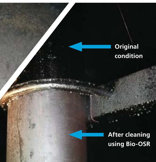
of FPSO heavy fuel oil tank before and after the cleaning with Bio-OSR
